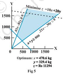
This gives the value of z as  $z = 10 \times 470.6 + 20 \times 329.4 = 11294$ This is the mathematical solution. **Step 4** The solution can be interpreted as saying that, "The minimum cost of the special food with corn and soyabean having the required portion of nutrient contents, protein and fibre is Rs 11294 and we obtain this minimum cost if we use 470.6 kg of corn and 329.4 kg of soyabean."
